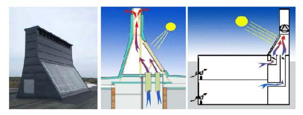
The chimney outlet should be located in a negative wind pressure zone. This negative pressure zone can be created by careful design of the roof profile and/or the chimney outlet. To provide adequate ventilation on very hot and still days, an extract fan can be installed in the shaft to pull air through the building. This should be designed so that the fan does not provide a significant resistance to air flow when the chimney is operating in its natural draught mode.
