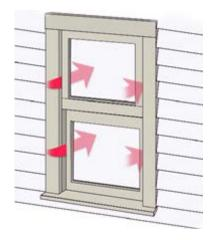
Air infiltration not only affects the building pressurization but may also distort the intended air flow pattern. Understanding infiltration requires understanding the pressures that cause the flow and the flow characteristics of the openings in the building shell.
