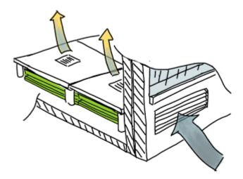
Ventilation inlets in the façade are often used in combination with local supply and extract of ventilation air. They need to have a certain size to support a sufficient air change rate with a low pressure-drop. Therefore, they influence the architectural expression of the façade. Local supply/extract of ventilation air does not need a special distribution system within the interior.
