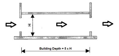
• The opening area required is approximately 2% of the floor area (1% on each side of the space).
