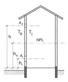
The height of the neutral pressure level, can be altered by changing the relative sizes (and/or number) of the upper and lower openings. If the upper opening is **increased** relative to the lower one, the neutral pressure level will rise. Conversely, larger openings towards the lower level will cause this height to fall.
