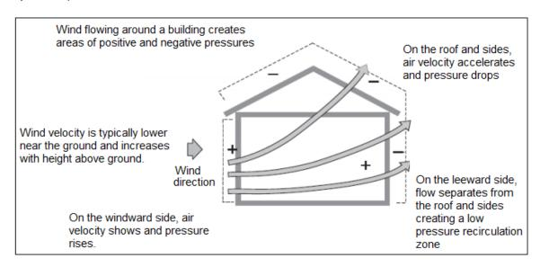
The magnitude of the wind pressure (P) is proportional to the velocity pressure, and is given by:
