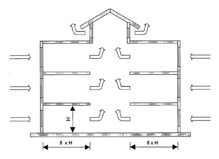
This rule is based on a building with a large stack or atrium running down the center of the building and spaces on either side of the stack having a maximum depth limit of 5 times the floor-to-ceiling height of individual levels. For example, a building with floor-to-ceiling height of 10 ft. on each level would be limited in depth to 50 ft. between the perimeter of the building and the stack. This results in a maximum depth building of 100 ft. plus the depth of central stack or atrium.
