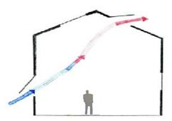
A key consideration when designing for Stack Ventilation is the location of inlet and outlet openings. The total amount of heat removed from a space is proportional to the height differential between the openings. In general, the greater the height difference between the inlet and outlet openings, the greater the volume of air pulled through the space, and the cooler the interior temperatures.
